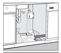
Certain steps in the installation procedures require that the dishwasher be pulled out of its opening. For this reason, perform the plumbing and electrical connections <u>after</u> the machine has been levelled and the front panel has been mounted.
